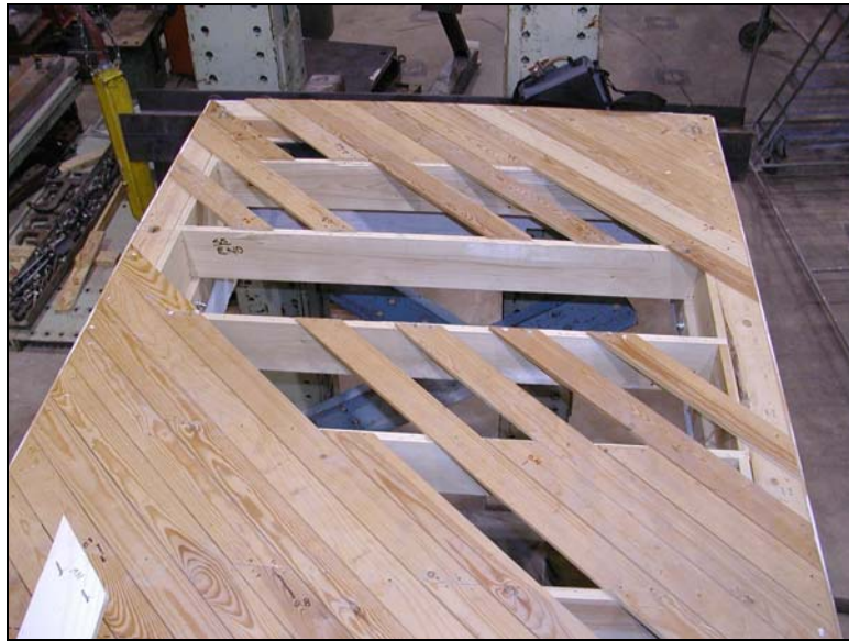
Figure 4.29 Strain-gauged sheathing boards removed and examined after testing
