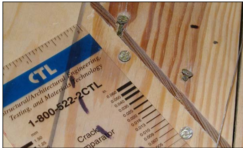
Figure 4.17 Nail withdrawal and tear-out at board end (DDR = 0.6 %)
