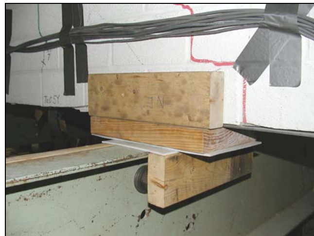
Figure 4.3 Low-friction bearing assembly between diaphragm and test frame
