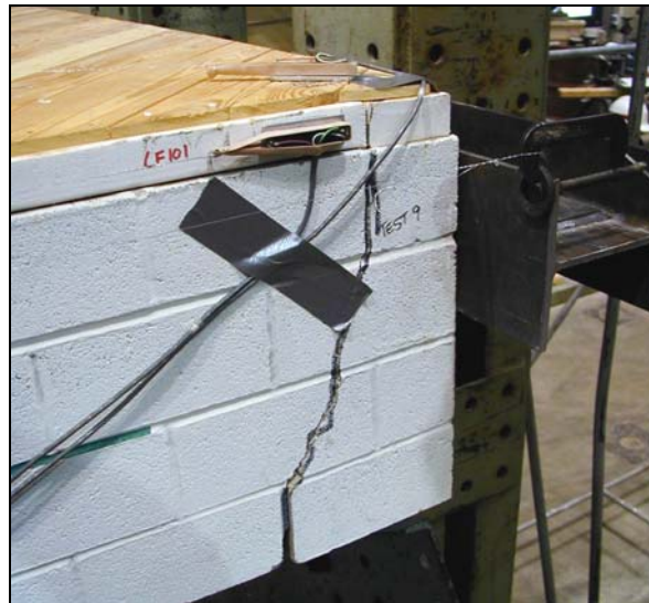
Figure 4.19 Sliding-shear failure during displacement to the west along pre-existing cracks in masonry chords (DDR = 1.1 %, northeast corner)
