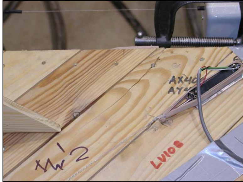
Figure 4.25 Longitudinal splitting of sheathing board at point of nailing (DDR = 1.5 %)
