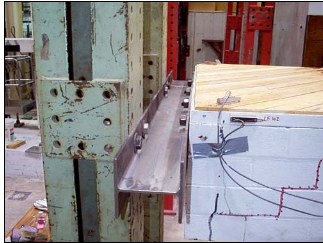
Figure 4.2 Box columns support south end of Diaphragm #1
